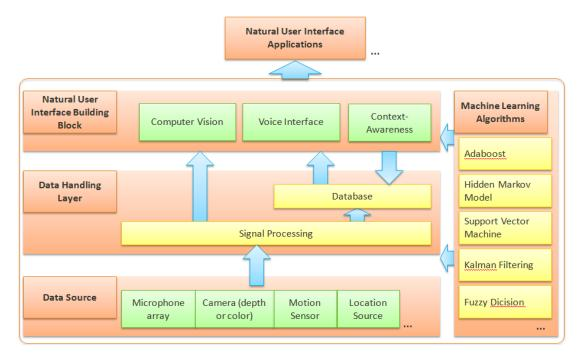
Figure 4. MediaTek Natural User Interface Software Framework
