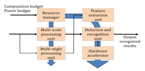
Figure 6. Computation and Power Budget Monitored and Dispatch by Resource Manager
